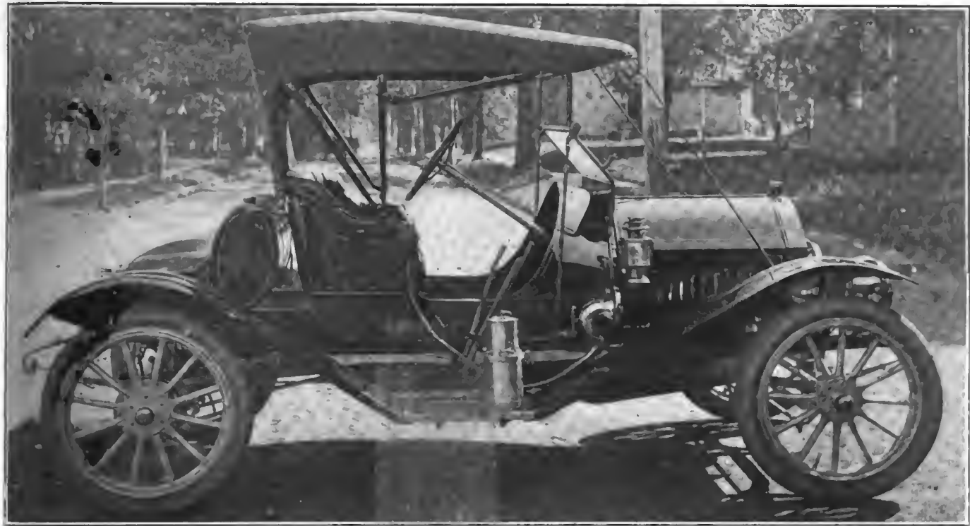
Model 25—Roadster, seating two persons, with an overhanging cowl, open entrance, commodious oval gasoline tank back of the seat and a tool box on the deck at the back
